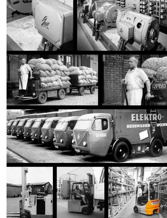
logically sophisticated STILL products with electrically powered drives available at present. Electric motors operate without couplings and gearboxes which is a fact that provides excellent driving comfort. Compared to internal combustion engines they are also characterised by low operation costs. Energy costs are lower as well as maintenance costs and their service life is longer. From his discussions with service customers Hans Still knew the weaknesses of the existing machines
